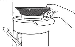
4. Place the juicer cover onto the juice collector/bowl, with the feed chute positioned over the stainless steel blade and filtering basket and push into position – figure 4.
